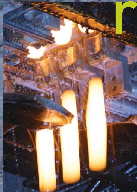
Molten glass being cut into 'gobs'
