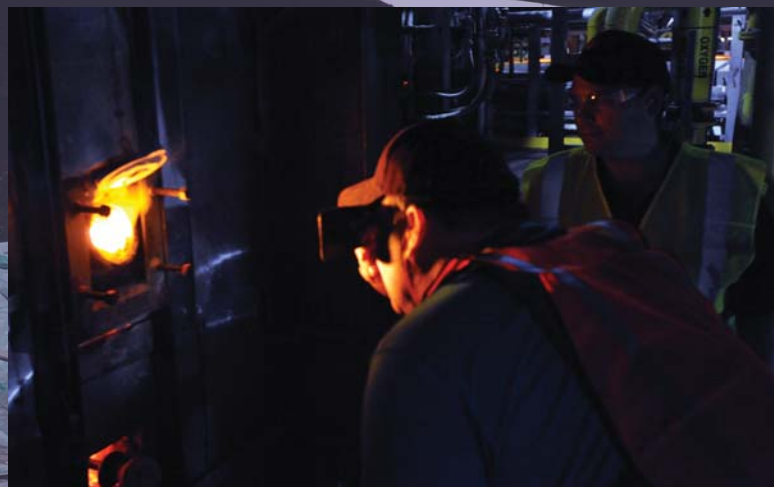
Molten glass is created at 2,850 degrees Fahrenheit
