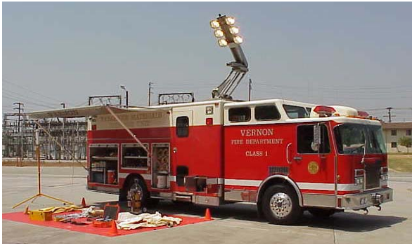
Hazardous Materials Emergency Response operate the Spartan Super Vac Hazardous Materials Unit
